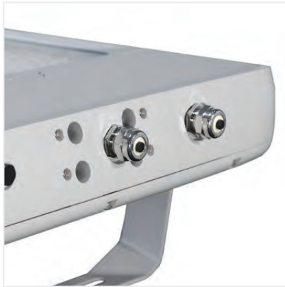
The floodlight includes two cable glands at the back (in and out) for a daisy chain layout. It is designed for integration with building management systems (DALI 2.0 or 1-10V protocol).
