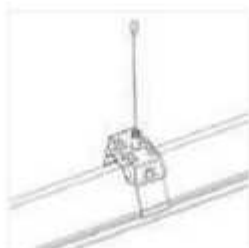
Suspension with ropes (roof version)
