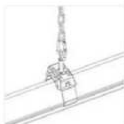
Suspension with chains (roof version)
