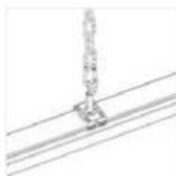
Suspension with chains (standard version)
