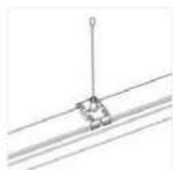
Suspension with ropes (standard version)
