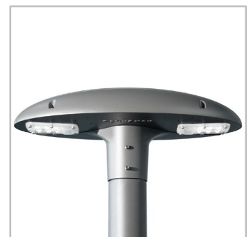
The luminaire is mounted on a Ø48-60mm spigot by tightening two M8 screws.
